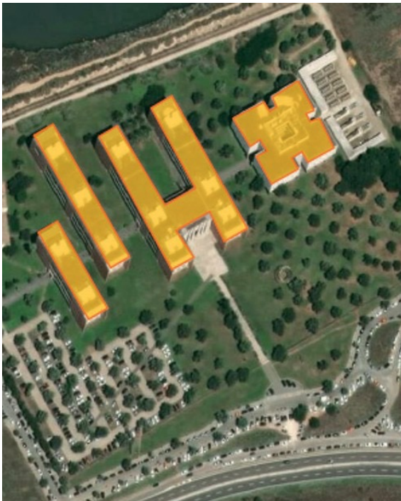
The image on the left illustrates the floor plan of the Sa Illetta site, showing the positioning of the photovoltaic modules (area colored in yellow). In the image above, the photovoltaic modules positioned are highlighted in blue.
